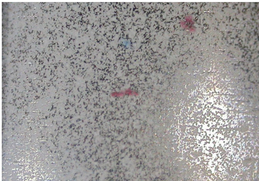
Figure 2 Small crack initiation in Alloy 690 steam generator tube; a dye penetrant indication.
