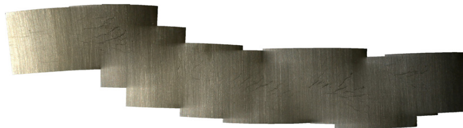
Figure 3 Circumferential cracking in steam generator tube samples.
